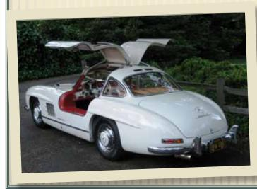
ixty years after its debut, this spectacular automobile remains undeniably one of the most beautiful ever built. Adding to its enduring appeal, the car is packed with innovative technology such as a slanted incline six-cylinder engine, fuel injection, a lightweight frame, and those iconic wing-like doors. As with many automotive advances, the 300 SL's groundbreaking features were developed from the marque's racing experiences. Built by Daimler-Benz AG,
